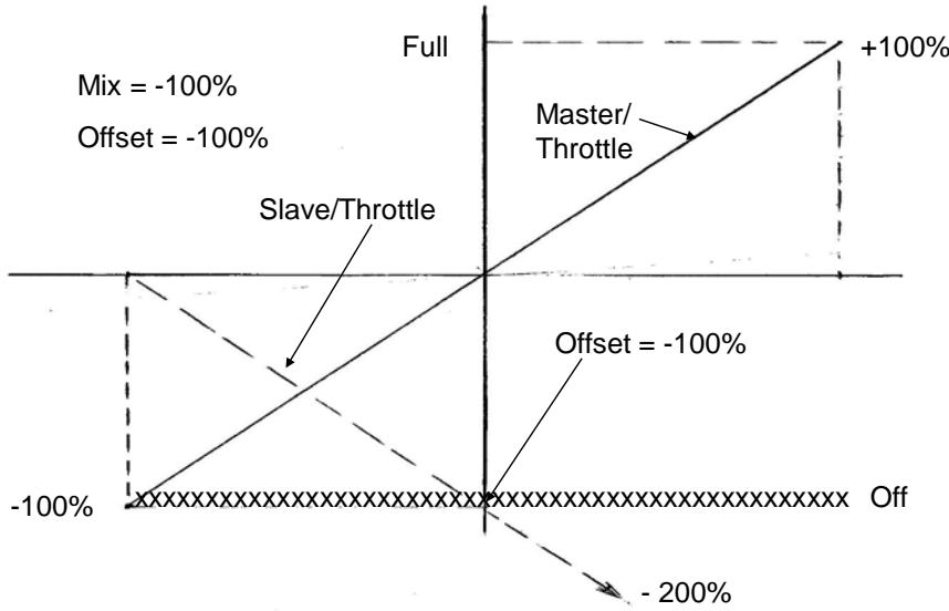
The offset function is used to modify the throttle channel response when the throttle cut function is activated (throttle to throttle mix is on).
