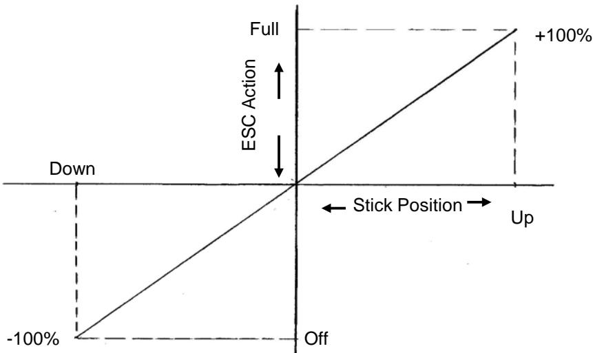
Slide 6 shows a typical throttle curve for an electric model. ESC action is substituted for servo rotation, but the operation is otherwise identical. Shown here is  $\pm 100\%$  throttle range. But my experience has shown that this programming procedure will work even though the range is not  $\pm 100\%$ . But, check it out before depending on it.
