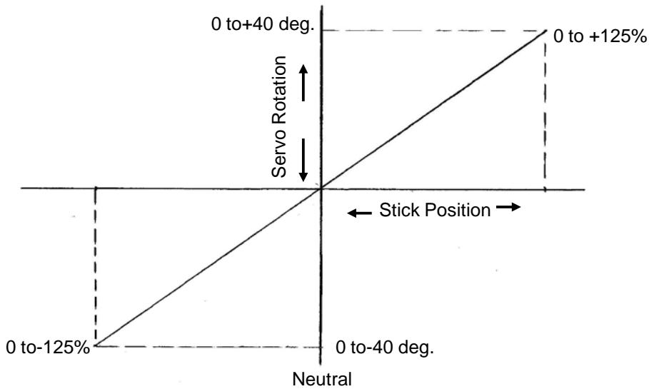
Slide 2 shows the servo response (typically up to 40 degrees or so) as a function of stick position. I will use servo response as the system output for this discussion even though (for electrics) there is no servo on the throttle channel. That way one can visualize what is happening in the throttle channel. The range of 0 to 40 degrees is shown because the transmitter can be adjusted to provide less servo response at the extremes than 40 degrees.
