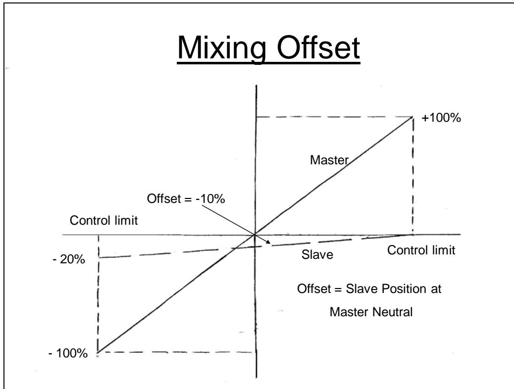
An additional mixing function is offset. Offset determines the slave channel position when the master channel output is at neutral (control stick center in most cases). This shifts the effect of the master on the slave. This feature is used in throttle cut programming.
