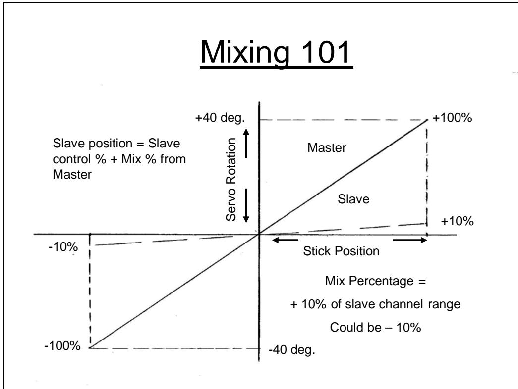
Mixing involves the interaction of two transmitter channels. The master and the slave. The master channel is typically the channel that controls the flying surface (rudder, aileron, elevator, etc.) The slave channel output is controlled by the slave channel controller (stick, switch, etc.) but is also controlled by the master channel when its position is changed. Also, in most cases, the master and slave channels are different, but not in the case we are considering.
